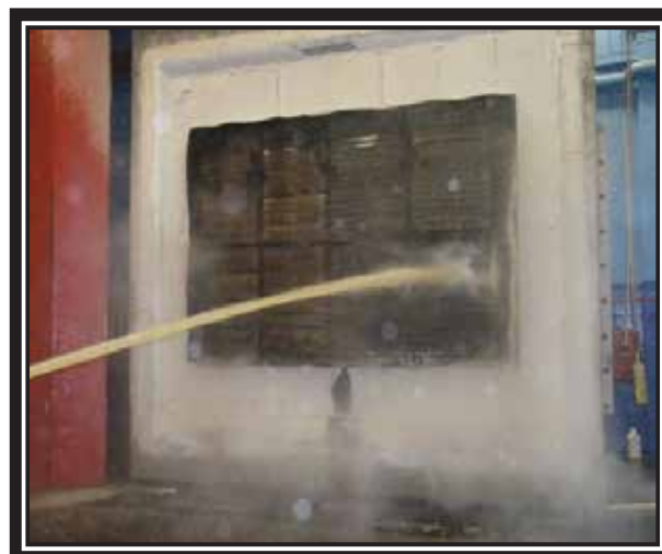
Hose Stream Test
